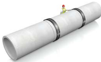
Slide coupling over one plain end.
