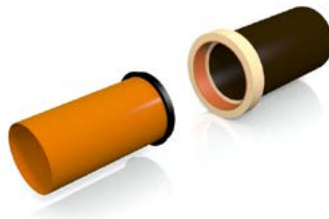
Apply lubricant to socket and Ü-P-Ring.
