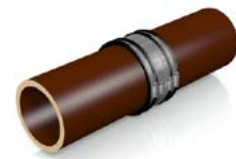
Center coupling over joint. Tighten clamps and shear band reciprocally.
