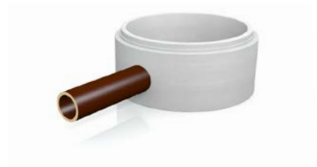
Push pipe into socket.
